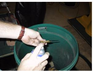
area. Wipe the excess oil away with clean dry cloth, put a drop of lubricating oil in the pivot area, open and close the knife a few times, and go show your wife.
