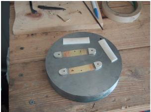
It's kind of hard to see what's going on in these next two photos. We need to drill through the backside of the liners and into the bone scales. This becomes difficult if the bone scales are thicker than the bolsters. If you don't drill the holes vertical, then the pins will not go through.
