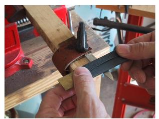
forth until all of the scratches in the blade go in one direction. Turn the blade around and do the same to the tang area. Flip the blade over and do the same to the other side. Then take the blade out of the vice
