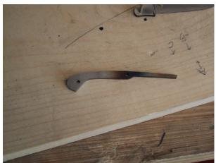
came out after going back through the heat treating, sanding, and tempering process. It's hard to see the blue color in the photo, but you should be able to see that the color is uniform from the tip to the center.
