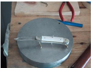
The knife looks pretty good at this point, but we need to grind the bolsters down and round them off. Take the knife apart and grind the bolsters by holding the liner.
