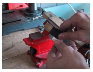
While the bone scales are drying, we will turn our attention to cleaning up the blade. Be patient and allow yourself plenty of time for these steps. I start off by clamping a board in the vice and c-clamping the blade to the board. I use leather around the blade to keep it from getting scratched up. Take a piece of brass, or any other flat and hard material, and wrap it with sandpaper. I start off with a 180 grit. Sand the blade back and
