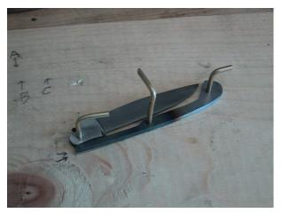
Close the blade and check to see if the tip of the blade needs to be lowered toward the spring. The tip of the blade will be raised a little when the spring under its load. I needed to bring the tip if this blade down a bit, so I ground a little from the tang at point C in the second photo. This brought the tip down as seen in the third photo. Be careful not to remove too much because you don't want the edge of the blade to be touching the spring.
