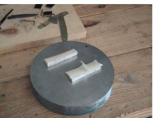
the bone. Grind the bone to the correct size against the grinder's flat platen. Hold on to the tab of tape like a handle.
