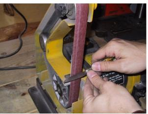
times to cut the main edge. Then I take it to a very fine stone and work it back and forth until I'm satisfied with the results. I'll also strop it to remove the wire edge. The knife is nice and sharp now.
