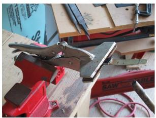
Heat the flux from the underside until it starts to bubble. Then put a small piece of solder in the corner and heat it form the underside as seen in the second picture. The solder will start flowing as soon as it heats up. Keep heating the underside of the liner until the heat pulls the flowing solder down around the bolster. Take a flux brush and brush the excess solder out of the corner.
