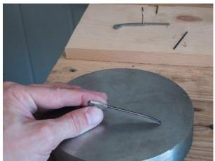
Now grind a 45 degree edge on each side of the blade down to the scribed lines. This will serve as your guide when grinding the rest of the bevels. To support the blade, I hold the tang with vice grips. I wrap a piece of leather around the tang to keep from scratching it up. Once you have your 45 degree edges ground, proceed to grind from the bottom edge to the black edge of the blade. Be careful not to grind past the back of the blade or the scribed lines at the edge.
