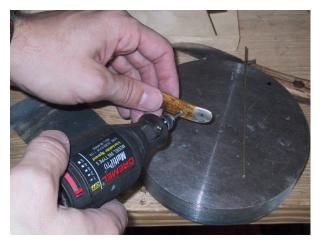
Once everything is dry, you will probably have to drill the holes in the liner again to remove the dried glue. Next, take a cone shaped Dremel bit and countersink all of the holes on the outside of the liners. You will also need to countersink the two small holes on the inside of the liners.
