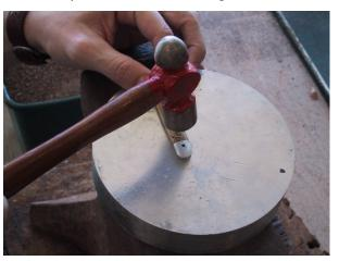
Take the side of the knife to the disk grinder and grind the edges of the pins down to about ½ as long as the pin is wide. Be careful not to let the disk hit the bone or the inside of the liner. With the peen end if the hammer, gently peen the ends of the pin down. The secret here is to go slow and
