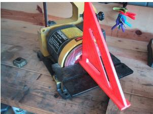
disk grinder's support table is square with the disk. Adjust the table if needed. Grind just enough from the inside edges of the bolsters to make them flat and smooth. Set these aside for now.
