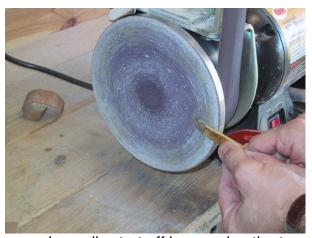
easy. I usually start off by peening the top surface. Then, as I peen the bottom surface, the peening will usually pull the head of the pin on the top surface nice and tight. Once you get the pins peened, flat sand the bottom of the liners to flatten the pin heads and to remove any super glue or scratches.
