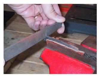
To make the tang longer, clamp the blade up in the vice. Using a safe edge file, file away. Be careful to only file forward and not to file down into the tang. The key here is to file a little, check it, file a little more, check it, ..... Keep doing this until the blade and spring fit up like in the second photo.
