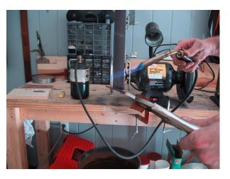
blue color should run uniformly from the end of the spring to just past the center hole. It's important to go past the hole so that the spring will not be brittle and week at its
