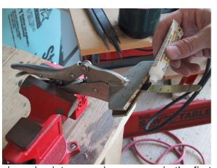
vice grips into your vice as seen in the first picture. Clamp a bolster to one end of a liner and put a drop of flux in the corner.
