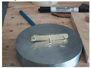
needs to be cut before heat treating. This will create scale down in the nail nick, and it will be black when the blade is completed.
