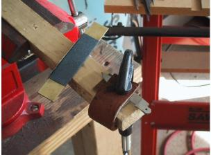
and sand the areas that you couldn't get to. When you have all of the scratches going in the same direction, go to a finer grit sandpaper and repeat the process but change the direction you are snading. Keep doing this until you get up to about an 800 grit paper. Be sure to remove all of the scratches from the previous paper before moving on to the next.
