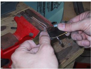
Put the knife together again and make sure that everything fits up and works correctly. Use nickel silver pins through the bolsters, and use a brass pin through the center of the spring. Cut the pins off as we did earlier, but you don't have to
