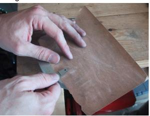
Place the blade between the liners and check to make sure that it lies evenly in the center. Make the necessary corrections if it
