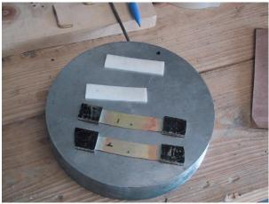
We now have our bolsters soldered to our liners. Grind the bolsters down to match the liner. Be sure to dip the liner and bolsters in water often to keep the heat down while grinding. It's very easy to overheat the bolsters and melt the solder. If this happens the bolsters will fall off, and you will have to go back and solder them again. Keep this in mind any time you are shaping or smoothing the bolsters. Flat sand the back of the liners and the top of the bolsters to remove any burs.
