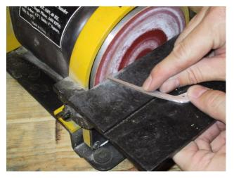
Grind a slight angle at the end of the spring. The angle should slope from the outside of the spring to the inside. (See the photo.) Only grind off enough of the spring to make a slight angle. Too much grinding will leave you with a short spring.
