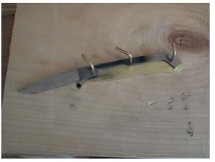
Place the liner with the holes in it on top of the solid one. Drill through the top liner and place a pin in each of the holes. Placing a pin in each hole after it is drilled
