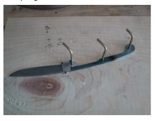
Now pin the blade and spring back on the board. Make sure that the back of the spring still lines up with the line that you made earlier. If it does not, just draw
