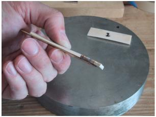
Clamp the liner and the second bolster up in the vice grips. Place the bone piece between the two bolsters and adjust the liner until the bone fits good and tight. Remove the bone and solder the second bolster. Clean up the solder joint with a
