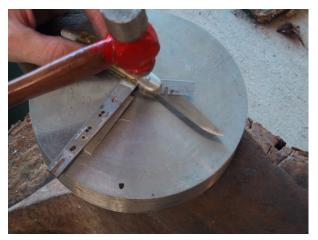
razor will keep us from peening the knife together and wedging the blade to where it will not open or close. Put the wedges in between the liners to keep the liners from closing up as we peen the blade in. Peen this pin like we did the other bolster. When finished, remove the wedges and the razor. The razor will be hard to remove, so be careful. I usually have to use pliers to remove it while I work the blade back and
