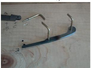
line. (See the arrows in the second photo.) Mark the wood where the back hole of the spring is now sitting. Drill this hole with a 3/32 inch bit and pin the spring to the board with both pins as seen in the second photo. This will create the load on the spring when the blade is pinned into place. Work the blade into place and put the pin in. It will be tight, but the spring should bend slightly allowing the blade and pin to be inserted.
