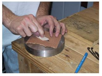
Throughout the process of making the knife, the knife pieces will need to be flat sanded to keep them smooth. Take a folded piece of tape and stick it to one side of the blade. Place a piece of sandpaper on a very flat surface, and rub the blade back and forth by holding on to the tab of tape. The goal here is to remove the burs left from grinding. I will refer to this process as "flat sanding" through out the rest of this tutorial. Flat sand both sides of the blade and the spring.
