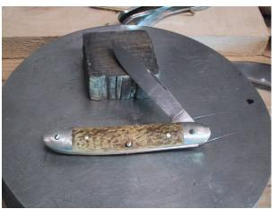
smack these pins with the hammer yet. The pins will stay in place because of the load on the spring. Take the knife to the disk grinder and grind the pins down to a length of about ½ of the pin's width. Peen the back and center pin down as we did earlier, but
