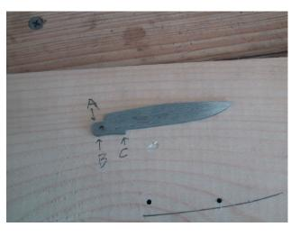
Take a black magic marker and color the bottom edge of the blade. Then place the blade on a flat surface and use a drill bit to scribe a line along the length of the edge. I use a 5/64 inch bit when working with a 3/32 inch blade. The line will be slightly off center. Flip the blade and do the same to the other side. You should be left with a thin solid black line in the center of the blade.
