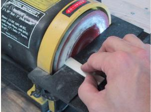
the bolsters. Also clean the sides of the bone up on the disk.
