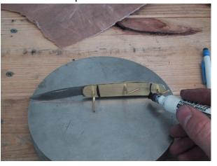
Now that we have the mechanical workings of the knife finished, it's time to turn our attention to making the sides. First decide how long the bolsters should be and draw them off on the liner. Color enough of the 1/8 inch Nickel Silver with the magic marker to allow you to scribe out four bolsters. Cut
