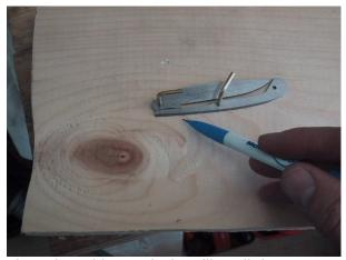
closed position, grind or file a little away from point B. This will lower the spring while the knife is in the closed position. Points A, B, and C are all tied in together. If you grind or file point B, the tip of the blade will rise from the spring. Therefore, point C will need to be filed or ground a little to bring the blade tip back down. Once every thing fits up correctly, it's time to grind the bevels into the blade.
