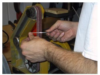
After I finish grinding with the 36 grit belt, I move to up to an 80 grit and bring the grind down to the scribed lines. You will notice that there are going to be a few places that will be hard to reach with the 2x72 grinder. I move down to the 1x30 grinder when I get to these places. I use files to clean up places that I can not get with the 1x30.
