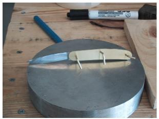
clamp two of the pins up in a vice. Use a Dremel tool with a cutoff wheel to cut the nail nick into the blade. If you want the inside of the nail nick to be black, than it
