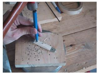
distance from the top to bottom to outside edge. Pin the bone and liner to a board with the center pin. Drill the first 1/16 inch hole and place a pin in it. Then drill the second hole. Placing pins through the holes as you drill them will keep everything lined up.
