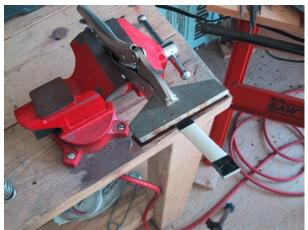
small triangle file until the bone fits nicely between the bolsters. Place the two liners back to back and put a pin though the center hole. You want to make sure that the bolsters on each side of the knife line up. Hold a bolster in place and mark the second liner with a pencil. Clamp the
