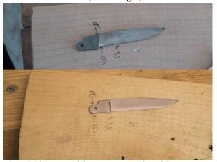
should be a golden straw color. You may have to adjust the temperature and time depending on your oven. I use to heat the blade at 400 degrees for an hour and a half twice, but the blades were coming out too dark. You can clean the straw color off the blade with a metal polishing compound or by sanding the blade again with a high grit paper.
