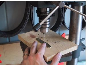
will help keep the liners lined up. The drill bit will leave sharp burs on the bottom sides of each brass piece. Flat sand these burs away before moving on.
