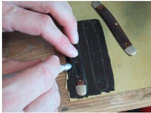
the shape of the original sides. I usually try to grind the pieces to between 1/8 to 1/16 inch outside of the scribed line as seen in the second photo. This gives me room to fit everything up. Flat sand the brass pieced to remove any burs from grinding.
