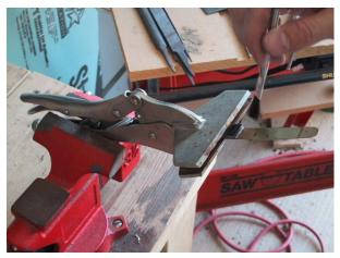
Check the solder joint to make sure that the solder goes all the way around the end of the liner. Add more solder to the joint if needed. Take a small triangle file and clean up the solder in the corner of the bolster and liner. You don't have to
