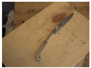
up grinding the tip of the blade off, so I had to go back and grind the spring so that everything would fit back up. Prior to heat treating the spring and tang of the blade need to be flat sanded to remove any burs. Flat sand each side of the spring as demonstrated before. You will not be able to flat sand the blade in the same manner because it is no longer flat. Rub both sides of the tang on the sandpaper as seen in the last photo. Do both sides, and take care to sand them evenly.
