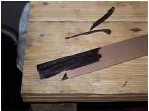
Use a metal cutting band saw to roughly cut the blade and spring out of the O1. If you do not have a band saw, a hacksaw will do the trick also. (It just takes longer.) Be sure to use a push block if you are cutting through pieces. It will be nice to finish the project with all ten fingers.
