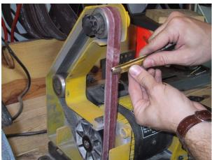
transition between it and the bolsters. The brass pins in the bone can also be ground down smooth if desired. When you are finished grinding, take a small file and round off all of the knife's edges. (Blade excluded.)
