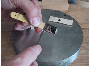
corner cleaned up, lay the bone piece against the bolster to make sure it fits. File more solder away from the corner if needed.
