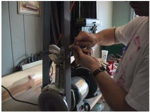
I use the flat platen to grid the bolster to their basic rounded shape. I then hold the liner and rock the bolster back and forth against a slack belt to round off the edges.
