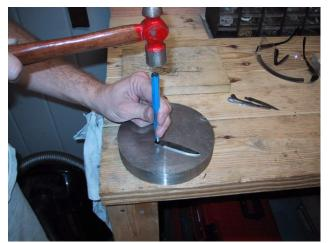
Using the old knife blade, mark the place where the pivot hole should go on the new blade. Note that the new blade will be slightly larger than the original. This is OK because we will have to make adjustments in the action of the knife by grinding areas away. You can always grind metal off, but you can never put it back. Use a center punch to pop an indention where the hole should be drilled. Go through these same steps with the spring.
