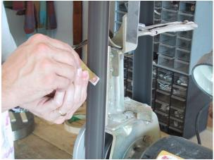
Turn one of the liners upside down and drill through each of the bolsters. Use the previously drilled hole in the liner as a guide. Put the knife together with pins to see how the holes line up. If you have trouble getting one of the pins through, take the assembled knife to the drill press and drill through the hole. This shaves off any edges that are keeping the pin from going completely through.
