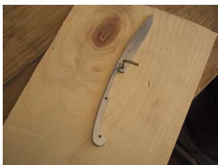
Next we must make sure that the spring of the knife will rest in the same position when the knife is both opened and close. An unfitted spring takes away from the beauty of the completed knife. First lay the blade and spring out like in the previous step. Make a mark onto the board at the place of the center pin hole. This will be the hole in the middle of the spring. Drill the hole out with a 3/32 inch bit and place a pin in it. With the blade in
