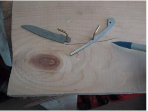
If the spring is lower than the drawn line when the blade is in the closed position, grind or file a little away from point A. This will lower the spring while the knife is in the opened position. You will need to redraw your line and check the open and closed positions again. If the spring is higher than the drawn line when the blade is in the
