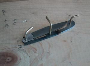
Now it's time to make the knife's liner. Take the black magic marker and color in enough of the 1/32 inch brass sheet to be able to scribe around each of the original knife's sides. Cut the brass pieces out with a band saw or a hacksaw and grind them close to
