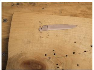
be softened a little so it's not so brittle that it breaks. Do this by heating it in the oven for 1 hour at 350 degrees. Take the blade out and let it cool to room temperature. Then put it back in the oven for another hour at 350 degrees. When the blade comes out it
