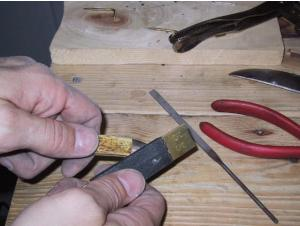
a mirror polished finish would. I sand up to about a 800 grit paper. Then I move to a "00" steel wool followed by a "0000" steel wool. This gives the bolsters, pins, and liner a nice smooth look, and it really polishes up the bone.
