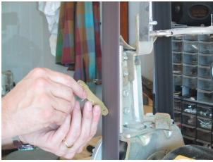
Take the knife apart, flat sand the liners to remove the burs, and put the knife back together. Open and close the knife a couple of times and see if you like the way the blade sits in the liners. If you don't like it, do a little more grinding and sanding on the liners until you like the way it looks. Once you are satisfied, take the knife and
