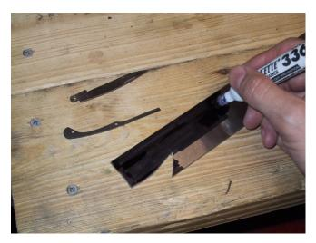
Take a black magic marker and color in enough of the O1 to allow the outline of the blade and spring to be scribed onto the steel. Using the old blade and spring as a pattern, scribe around each.
