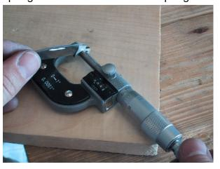
just under .094 inches. I usually try to bring the sides of the tang down to around .085 inches or so.
