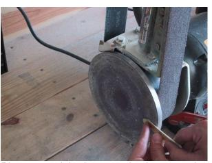
Place one of the bone scales between the bolsters of a liner. Use the disk grinder to bring the surface of the bone down to the height of the bolsters as seen in the first photo. Now the bolsters and bone will line up when placed upside down on the drill press as seen in the second photo. Drill a
